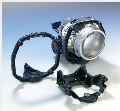
Drive unit for curve-following light
